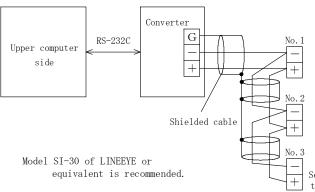
In case of RS-485 connection, up to 32 devices, includes the upper computer, are possible to connect. Specify the end station for both ends of device on the line. Set the terminator to be short-circuited for the identification of the end station. Lead wire for short-circuit is not attached. Use the converter for another identification to set the terminator.
