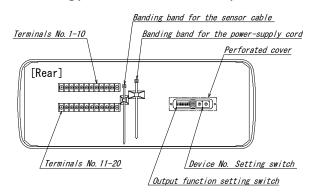
Terminals No.11-15: I/O terminal for RS-232C and RS-485. Output function setting switch: Set several functions for serial communication.
