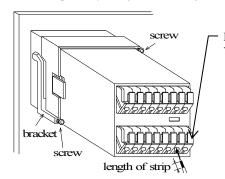
Push this portion (lever) to insert the wire for connection. You can directly insert hard single-wire without pushing
