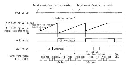
NOTES 3: In case of the total reset function is disable, automatically resets the total to zero and frequency dividing of P.O. output goes clear.
