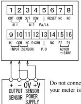
Do not connect to the terminal 11if your meter is not supplied the sensor power.
