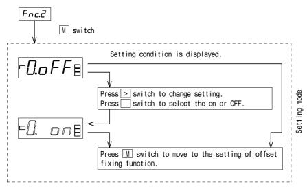
When the zero set function is made to be able and the zero set terminal is short-circuited to the COM terminal, the display becomes the offset value (the value set at the article 3.2.1)
