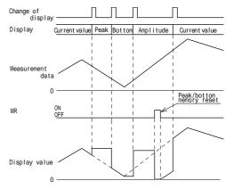
When the MR input terminal is ON, the memory data is continuously updated, so the current value is displayed and output. In case of amplitude, however,
