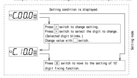
Adjustable range: 00.0~19.9%, however, the cut-off function is disabled when 00.0 is set. Adjustable range for the AC input models is 00.1~19.9%.
