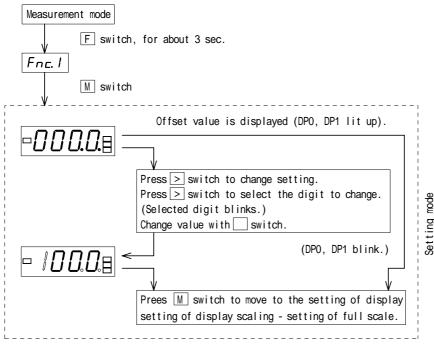
Offset value display means the display at the input of  $0mV(V, \mu A, mA, A)$ .
