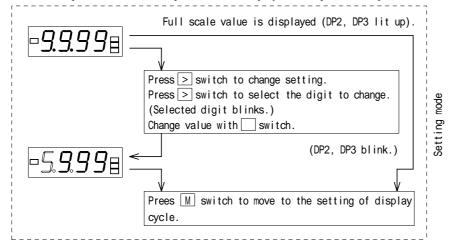
Full scale display means the display at the input of max. value of the rated input.
