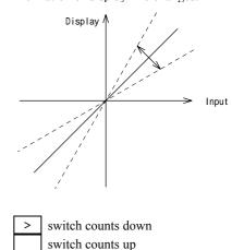
When the scaling width is narrow, It takes some time to start count. Keep pressing the switch for a while.
