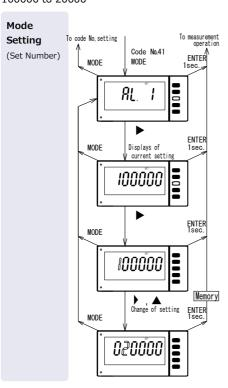
AL3 to 4 totalized value alarm output, change of batch output totalized value alarm output can switch to upper limit and upper limit alarm output or totalized value batch output.
