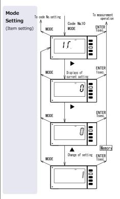
Function mentioned above are the main setting methods. The setting of the other operation methods are also like the setting method of the code No.00 to 03 and No. 06 to 10. The detail description of the setting ranges are omitted here. Please perform the other setting when necessary referring the Function code list mentioned on page 16.
