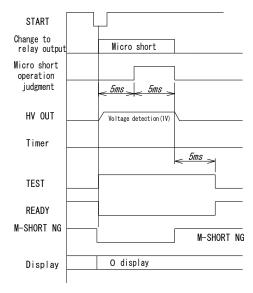
• During withstand voltage NG judgment after Micro short test
