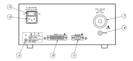
HIGH VOLTAGE terminal High voltage terminal where output of High voltage is obtained during test.
