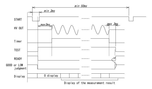
When test mode is in MANUAL CRL mode and if NG judgment is obtained, test can't be done by start signal. Releasing the NG judgment (OFF) by STOP signal, input the START.
