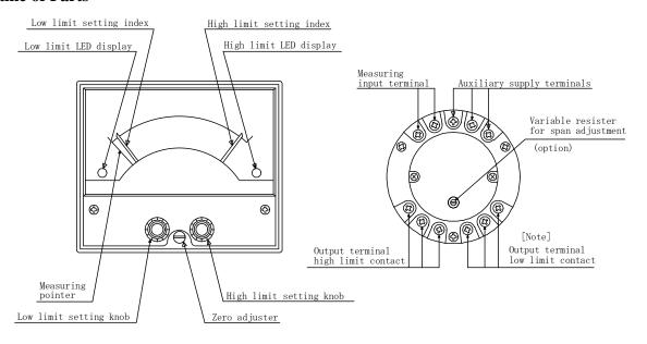
**Note:** In case that the model name is NRC-120H, no low limit setting lever, set point index bar ,low limit display or contact output terminal is provided.
