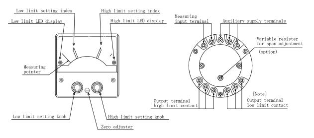
**Note:** In case that the model name is NRP-83H, no low limit setting lever, set point index bar ,low limit display or contact output terminal is provided.
