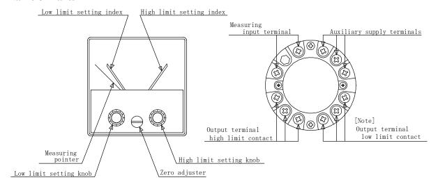
**Note:** In case that the model name is NRP-60H, no low limit setting lever, set point index bar ,low limit display or contact output terminal is provided.
