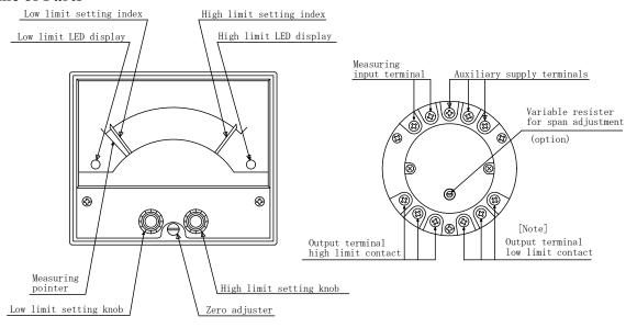
**Note:** In case that the model name is NRC-100H, no low limit setting lever, set point index bar, low limit display or contact output terminal is provided.
