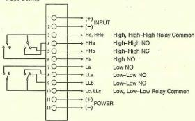
Note: Indicator type has the input and the aux. power terminals only.
