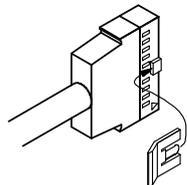
Connect the measuring cable (option) to the measurement connector on the rear panel. The measuring cable is capable of 5 channels, so in order to measure the 20 channels, you need to connect all the 4 cables.
