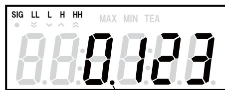
The decimal point location is determined as specified in the parameter setting P08.
