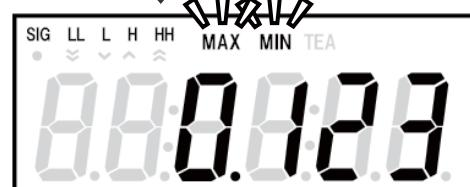
Press and hold the **MEM** key for 5 seconds during the normal measurement or when the maximum/minimum value is displayed, the MAX and MIN lamps blink for 2 seconds.
