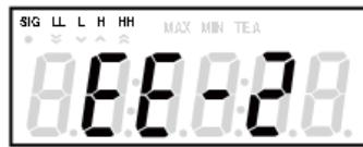
Displays "EE-2" for a second, and then returns to the normal measurement display.
