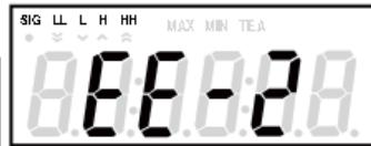
Displays "EE-2" for a second, and then returns to the normal measurement display.
