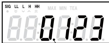
The decimal point location is determined as specified in the parameter setting P08.
