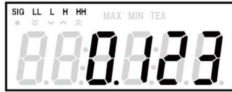
After the MAX and MIN lamps blink for 2 seconds, the memory is cleared and the display returns to the normal measurement display.
