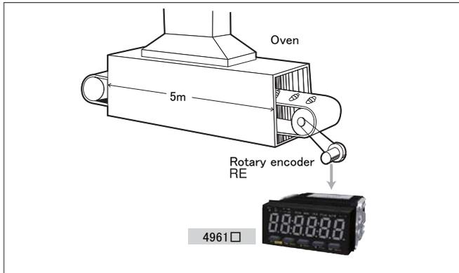
As in the figure on the left, bread passes through the oven in a bread factory. The rotary encoder is attached to the motor of the conveyor belt. To display the time at which the bread passes through the oven in 4961□, do so under the following conditions:
