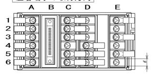
推奨圧着端子: V1.25-FS3(冨士端子工業製)
