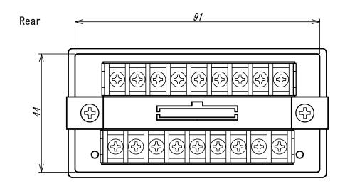
Panel cut-out dimension  $92^{+0.8} \times 45^{+0.6}$ Terminal screws : M 3
